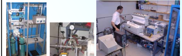
Fig. 5: Illustration of the vertically aligned nanotube chemical vapor deposition growth plant. (a) Gas mixture control cabinet. (b) Vacuum seal and pressure gauge. (c) Panoramic view of part of the plant.
