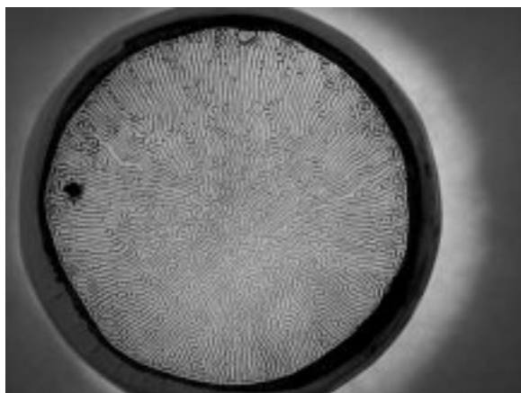
Figure 4. Labyrinth instability that results when a 1 mm thick layer of ferrofluid between 4 inch diameter glass plates is stressed by a magnetic field of about 250 G tangent to the thin dimension of the ferrofluid layer.
